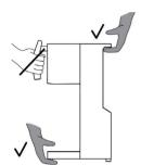
Hold the Carrying grip  $(\underline{1})$  and Carrying handle  $(\underline{7})$  to lift the MINI 96.
