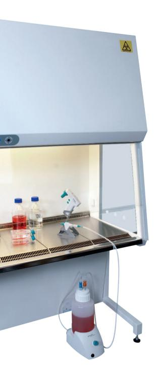
Vacuum systems are widely used for aspiration of liquids and their subsequent disposal. Common applications include the removal of media from cell cultures, of supernatants after centrifugation and of wash solutions from immuno-assay well-plates.
