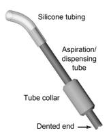
The aspiration/dispensing tubes delivered with the DOSE IT facilitate the dosing process and are fitted on the end of the tubing. The aspiration tube is dented on one end in order to guarantee a free flowing of the liquid entering the tubing. Make sure not to insert the dented end of the aspiration tube into the silicone tubing.
