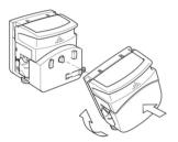
3 Assemble the two pumpheads by locking the original pumphead onto the extension pumphead. When turning the original pumphead in place, ensure that the lock mechanism engages with an audible click.
