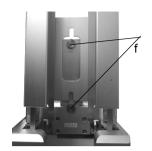
Connect the stacker chimneys by lowering them over the pins (f) on the chimney support brackets.
