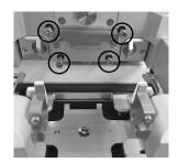
Align and attach with four hex screws. Make sure the cable is not pinched between the stacker and the assembly.
