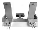
From the back of the stacker put the support brackets on the top of the Stacker Base and pull them to their stop.
