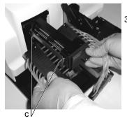
3) Hold the black left and the right dispensing cartridge below the rollers of the pump head, so that the tubings points downwards and the screws upwards. Fit the two holes on the inside of the left cartridge (28) with the two silver pins (c) located on the sliver lever. Position an equal number of tubes in front of and behind of the middle black roller wheel (25).
