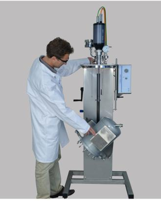
10 liters kiloclave, 60 bar, 200 °C non-EX stirrer drive (ceramic) Tantalum gasing stirrer
