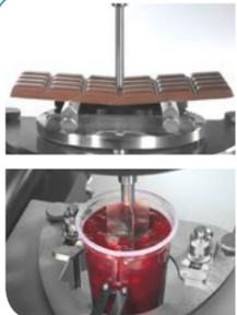
Texture analysis of solid samples with fixtures for bending, breaking or squeezing tests
