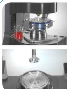
Electrical temperature module for parallel plates with active upper heater for tests up to 400 °C
