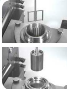
Large dimension building material cell with exchangeable lamella profiles
