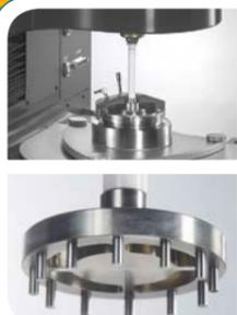
Variety of sample covers including solvent trap to minimize solvent evaporation
