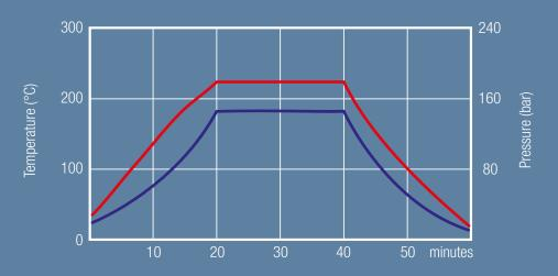
Typical ultraCLAVE digestion cycle with the 40 position rack. 0.5 g of organic samples such as infant formula, butter an API and fish oil with 5 mL of HNO
