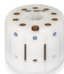
SK-10/12 High-pressure digestion rotor
