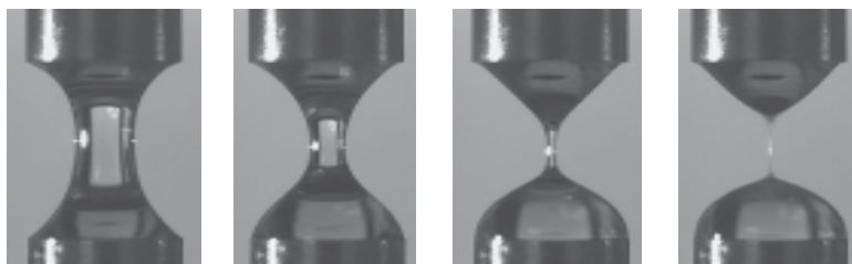
Figure 2: Sequence of a CaBER measurement [1].
