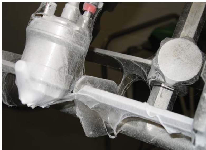
Fig. 1: "Cobweb" caused by filament formation.
