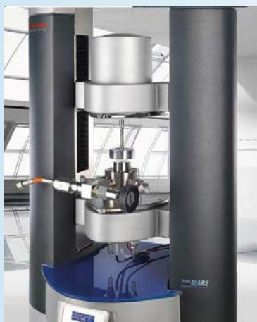
HAAKE MARS with high pressure measuring cell
