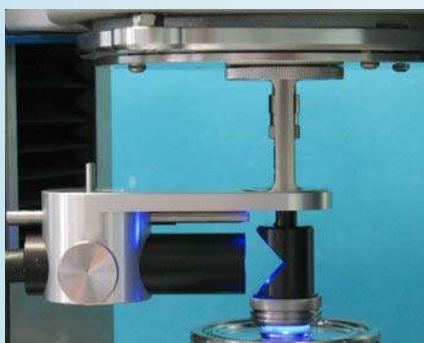
Measuring cell for thermal assisted UV curing
