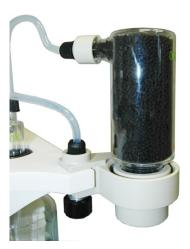
Fig. 5.16: Adsorption vessel with activated charcoal and glass wool
