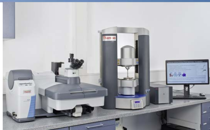
Fig.1: Combination of a HAAKE MARS rheometer with RheoRaman module and adapted Nicolet DXR Raman microscope.
