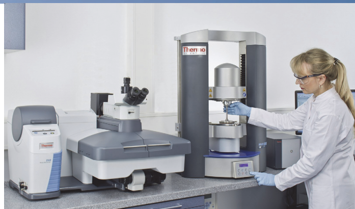
Fig. 1: Combination of a Thermo Scientific HAAKE MARS with a Thermo Scientific DXR Raman Microscope.
