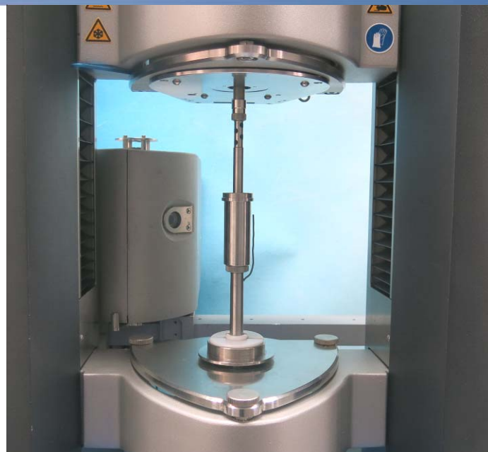
Fig. 2: Z20 DIN for CTC geometry in measuring position with temperature sensor.
