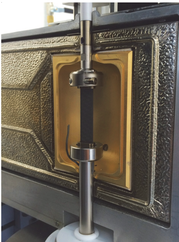
Fig. 2: Solids clamping tool with carbon fibre enforced composite sample.
