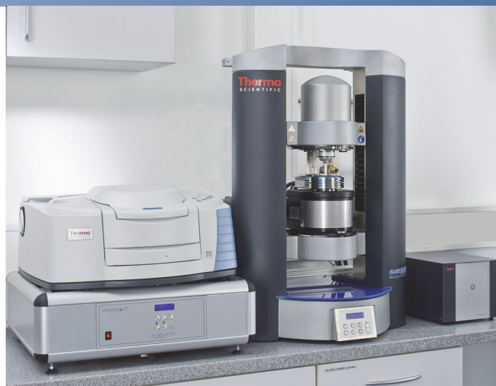
Fig 1: Setup with HAAKE MARS rheometer, Rheonaut module* and FT-IR spectrometer.
