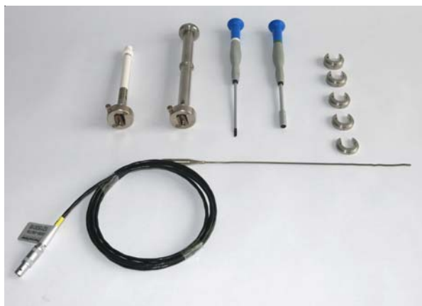
Fig.4: Solids clamping tool with temperature sensor, spacer and tool.
