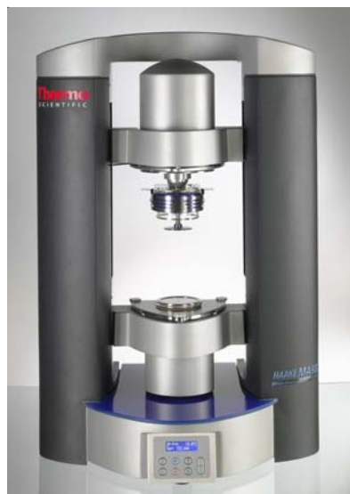
Fig.3: Detail view of HAAKE MARS Rheometer with RheoRaman module and upper temperature module TM-EL-H for high temperature application.
