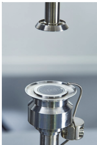
Fig.3: Detailed view - parallel plates geometry with integrated DEA comb sensor.
