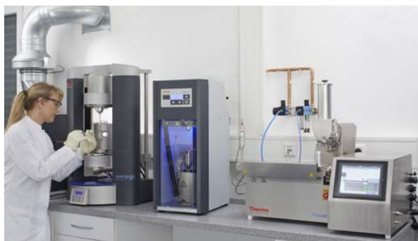
Fig. 2: Polymer workflow (from right to left) Mini compounder, injection molding system to produce test specimens and HAAKE MARS 60 rheometer with controlled test chamber for polymer tests in a temperature range between -150 °C up to 600 °C.
