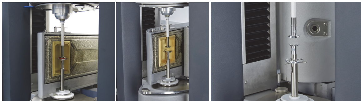
Fig.3: HAAKE MARS with Controlled Tests Chamber (CTC) half-open (left); Standard measuring geometry for CTC consisting of lower shaft with exchangeable plate and upper rotor with ceramic shaft (middle); Disposable measuring geometry for CTC with collection device to prevent chamber fouling (right).
