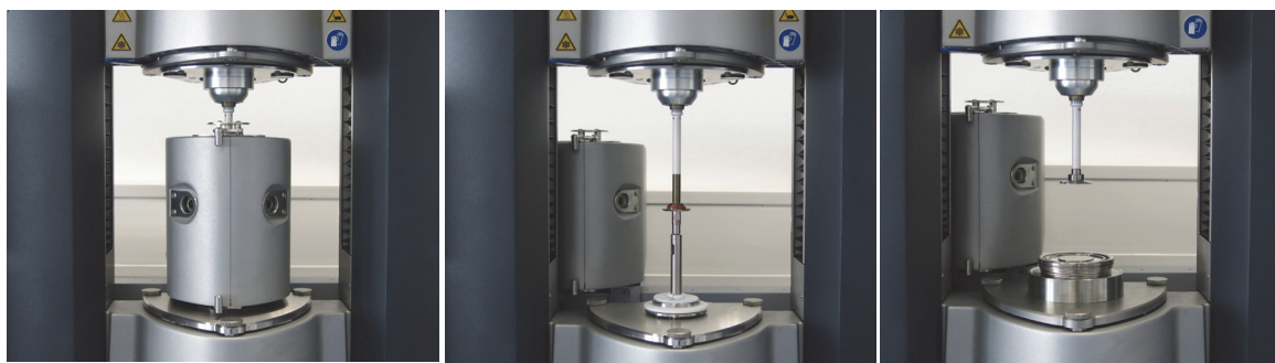
Fig. 2: HAAKE MARS with Controlled Test Chamber (CTC) in measurement position (left); in parking position (middle); in parking position and Peltier temperature control modules for parallel plates and cone & plate mounted (right).
