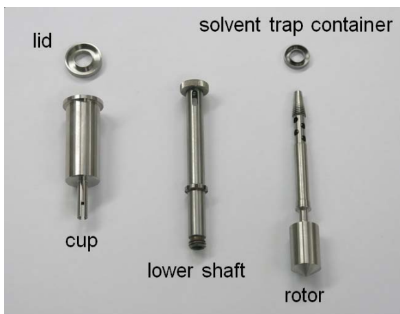
Fig. 1: Individual parts of Z20 DIN for CTC measuring geometry.
