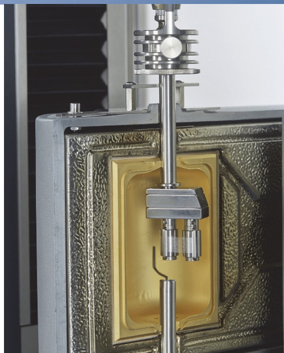
Fig. 1: Controlled Temperature Chamber (CTC) of the HAAKE MARS with the SER.
