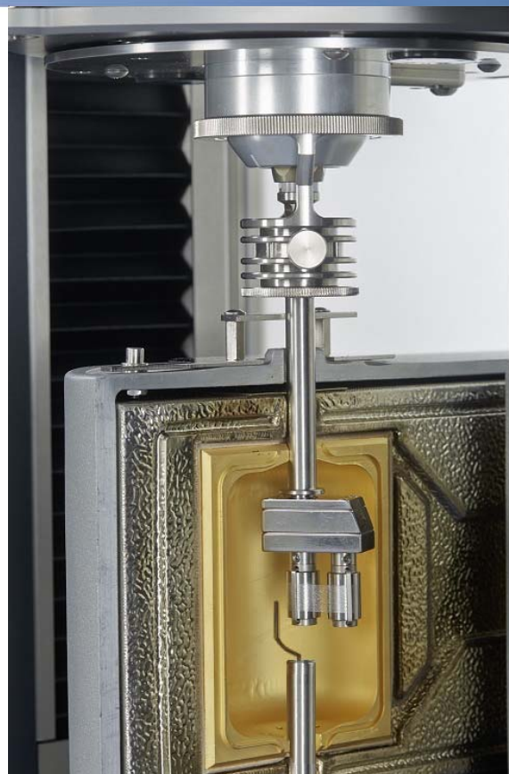
Fig.1: SER3 tool with HAAKE MARS rheometer and Controlled Test Chamber (CTC).
