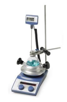
Comes complete with a 250 ml base, heat resistant lifting handles and a 100 ml flask adapter
