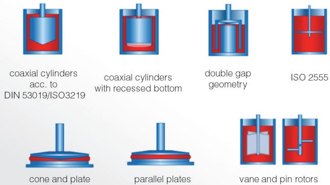
**Fig. 1:** Overview of standard measuring geometries.
