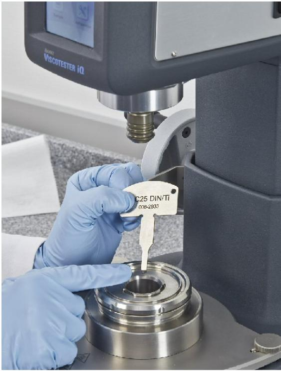
Fig. 4: Level gauge for coaxial cylinder geometries.
