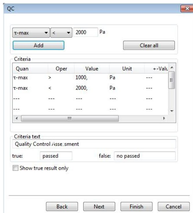
Fig. 7: Definition of QC criteria in HAAKE RheoWin software.
