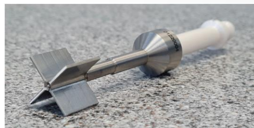
Figure 3: 4-blade vane rotor used to simulate cutting or biting the product.
