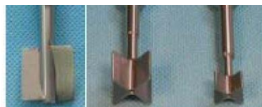
Fig. 2: Propeller shaped 2-blades vane rotor FL26-2b with fitted shaft adapter (left) and 4-blades vane rotors FL22 and FL16 with shaft adapter (right)
