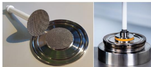
Figure 2: Upper and lower serrated plate (left) and measuring geometry with cheese sample (right).
