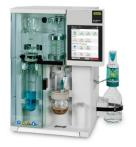
KjelMaster K-375 Steam distillation and titration
