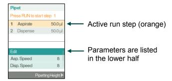
Insert the GripTips into the liquid to be transferred. Press and release the **RUN key** to aspirate the volume selected in the first step.
