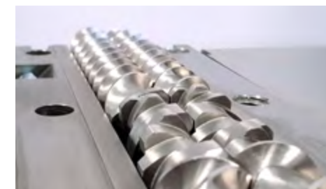
The B-TSE-S 30/40 features an electrically openable liner for optimum process monitoring and easy cleaning
