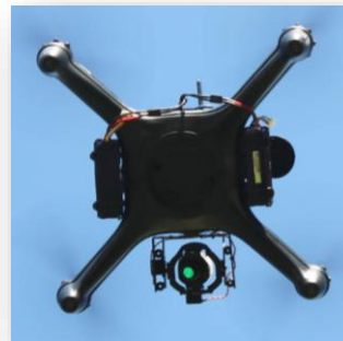
OCI™-D2000 system on gimbal during flight
